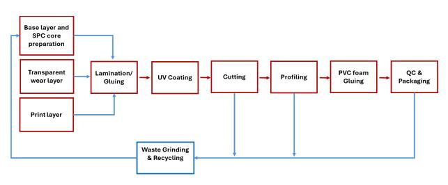
Figure 2. Production Process of Kährs LVT SPC Click with PVC Foam Underlayment
